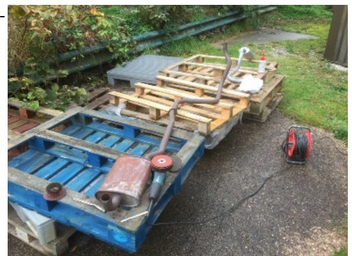
Original Ford exhaust was bead-blasted, plated and sprayed by Andy while the body shell was away being painted.
