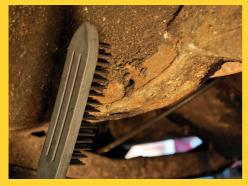
**PREPARE THE SURFACE** As with any topcoat, the quality of the final result depends on the quality of the preparation. Remove any loose or flaking rust using a wire brush.
