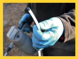
**THE IDEAL TOOL FOR THE JOB** The smaller probe can be attached so that Waxoyl can be applied to the internal surfaces of box sections and other areas in which a cavity wax offers best protection.
