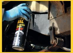
**SPRAY IT ON FOR FAST RESULTS** For larger external surfaces, such as this chassis member, use Hammerite Underbody Seal aerosol. Ensure that you are wearing a mask, and work in a well-ventilated area.
