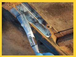
**TREATING SURFACE RUST** After using the wire brush to remove any loose material, apply Hammerite Kurust rust converter to all remaining surface corrosion and allow it to dry.
