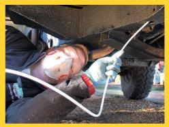
**PROTECTING INTERNAL SURFACES** Insert the extention probe into the box section, then smoothly withdraw it as you spray. The new nozzle gives excellent 360° atomisation for maximum coverage.
